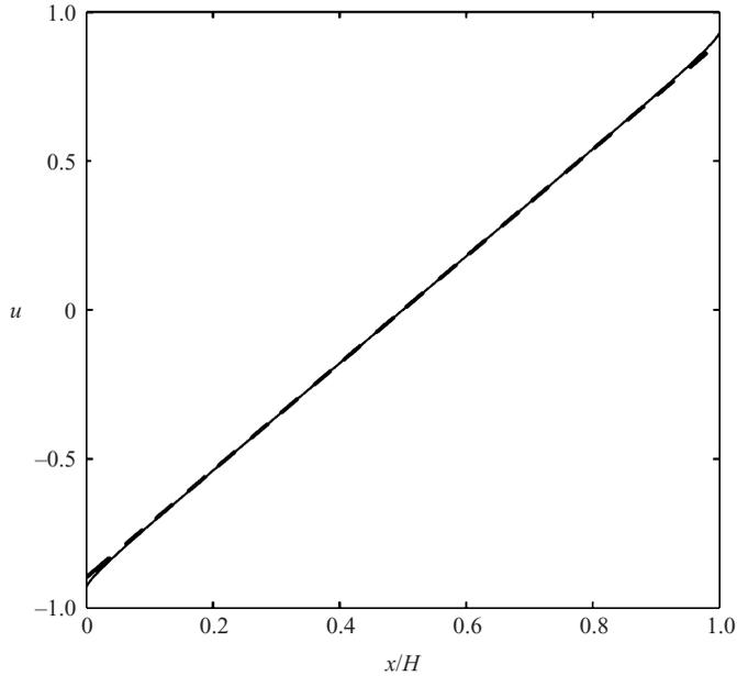
FIGURE 9. Non-dimensional velocity profile for Couette flow,  $Kn = 0.05$  ( $= \lambda/H$ ). Comparison of the BGK solution (—) with the slip solution (---). Non-dimensional wall velocities at  $x = 0$  and  $x = H$  are  $-1$  and  $1$ , respectively.
