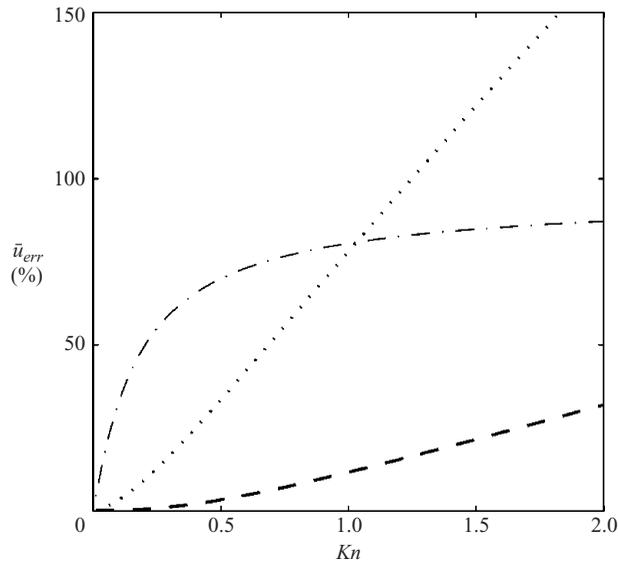
FIGURE 15. Average error of Poiseuille flow velocity predictions up to  $Kn = 2.0$ . Comparison of no-slip solution ( $- \cdot -$ ), slip solution ( $\cdots$ ), and our model ( $- - -$ ). The non-dimensional applied pressure gradient is  $Kn$ .
