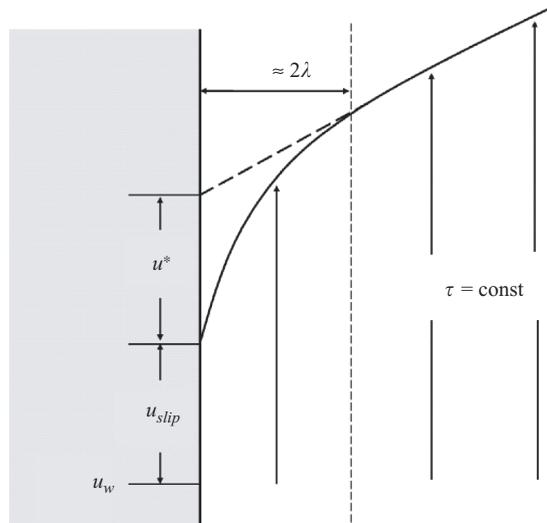
FIGURE 8. Schematic of the Knudsen layer extending out from a solid wall surface (shaded):  $u_w$  is the velocity of the wall;  $u_{slip}$  the velocity slip at the wall;  $u^*$  is the amount of ‘fictitious’ slip velocity that would be required to ensure that a Navier–Stokes solution (diagonal dashed line) provides an accurate prediction (solid line) beyond the Knudsen-layer limit (vertical dashed line).
