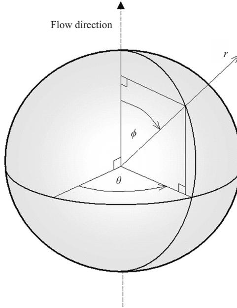
FIGURE 19. Coordinate system for the micro-sphere flow problem.
