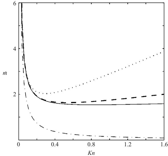
FIGURE 16. Normalized mass flow rate predictions for Poiseuille flow up to  $Kn = 1.6$ . Comparison of no-slip solution ( $- \cdot -$ ), slip solution ( $\cdot \cdot \cdot$ ), BGK solutions ( $-$ ), and our model ( $- -$ ). The non-dimensional applied pressure gradient is  $Kn$ ; the non-dimensional mass flow rate is normalized with  $\sqrt{\pi}/(2Kn)$ .
