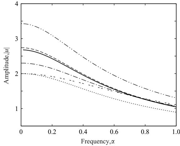
FIGURE 4. Wave-amplitude variation with non-dimensional body-force frequency,  $\alpha$ ;  $Kn = 0.5$ . BGK solution (—); Navier–Stokes ( $\cdots$ ); Burnett (---); super-Burnett ( $-\cdots-$ ); Grad's 13-moment ( $-\cdot-\cdot-$ ); regularized 13-moment ( $-\cdot-\cdot-$ ).
