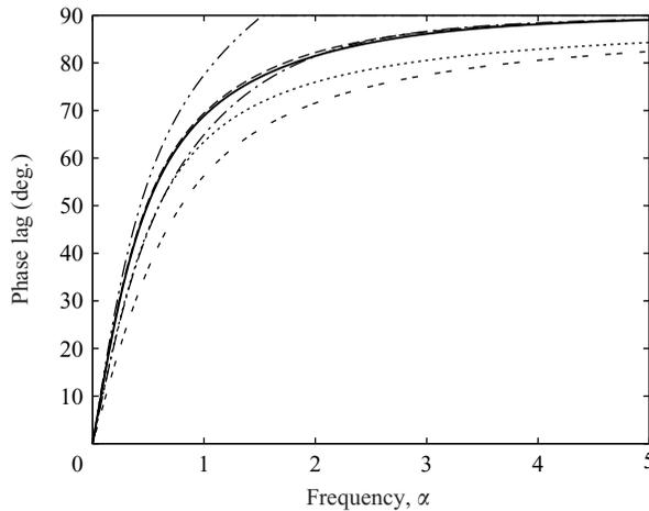
FIGURE 5. Velocity-phase-lag variation with non-dimensional body-force frequency,  $\alpha$ ;  $Kn = 0.5$ . BGK solution (—); Navier–Stokes ( $\cdots$ ); Burnett (---); super-Burnett ( $-\cdots-$ ); Grad's 13-moment ( $-\cdot-\cdot-$ ); regularized 13-moment ( $-\cdot-\cdot-$ ).
