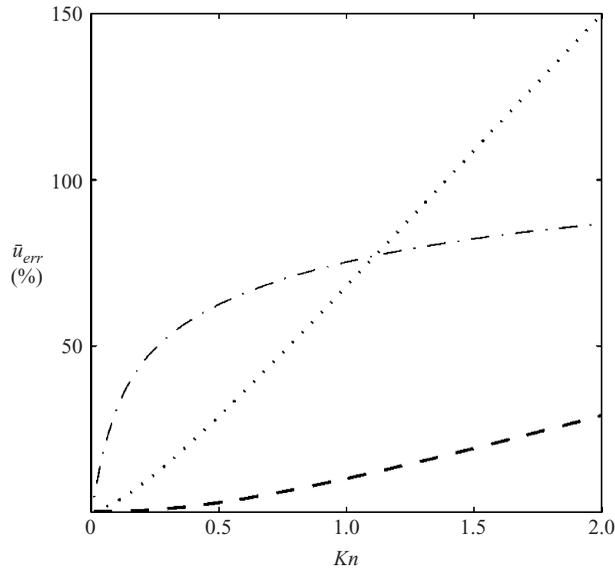
FIGURE 18. Average error of combined Couette/Poiseuille flow velocity predictions up to  $Kn = 2.0$ . Comparison of no-slip solution ( $- \cdot -$ ), slip solution ( $\cdots$ ), and our model ( $- - -$ ). The non-dimensional applied pressure gradient is  $Kn$ .
