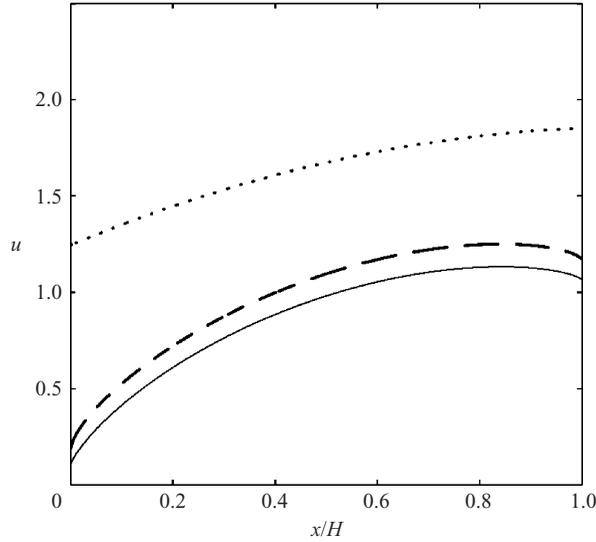
FIGURE 17. Non-dimensional velocity profile for high-Knudsen-number combined Couette/Poiseuille flow ( $Kn = 1.0$ ). Comparison of the slip solution ( $\cdots$ ), the BGK solution ( $-$ ), and our model ( $- - -$ ). The non-dimensional applied pressure gradient is  $Kn$ , and the non-dimensional wall velocities at  $x = 0$  and  $x = H$  are  $-1$  and  $1$ , respectively.
