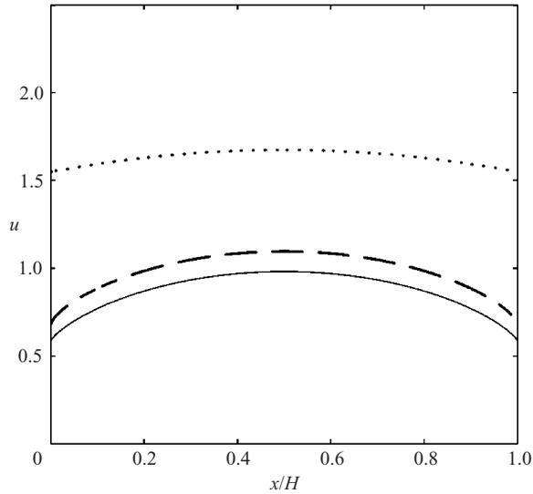
FIGURE 14. Non-dimensional velocity profile for high-Knudsen-number Poiseuille flow ( $Kn = 1.0$ ). Comparison of the slip solution ( $\cdots$ ), the BGK solution ( $—$ ), and our model ( $- - -$ ). The non-dimensional applied pressure gradient is  $Kn$ .
