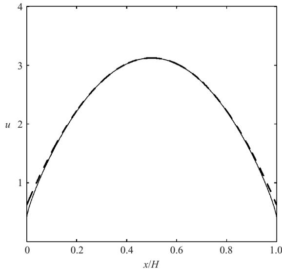
FIGURE 10. Non-dimensional velocity profile for Poiseuille flow,  $Kn = 0.05$  ( $= \lambda/H$ ). Comparison of the BGK solution (—) with the slip solution (---). The non-dimensional applied pressure gradient  $= Kn$ .
