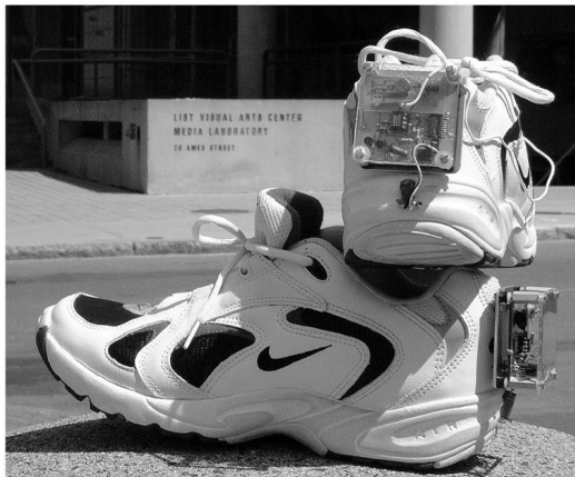
(a) Piezoelectric-powered RFID shoes with mounted electronics
