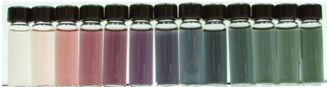
Figure 4.9. Colloidal solution of gold nanoshells showing a spectrum of color corresponding to different stages of shell growth and thickness of gold shell. Generally, as the shell grows on the silica core, the color changes gradually as shown in the direction from left to right.
