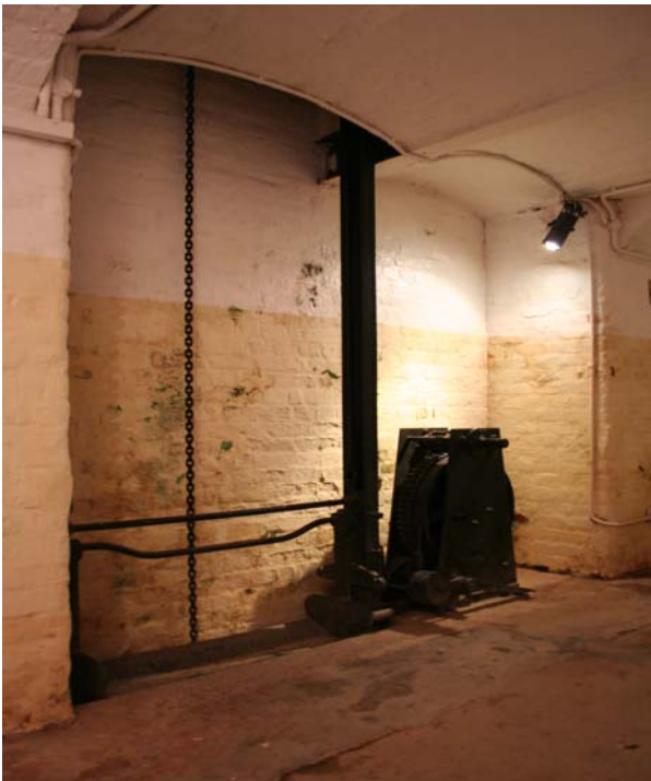
Illustration 35. A surviving example of the mechanical shell hoist at Fort Siloso. (Author)
