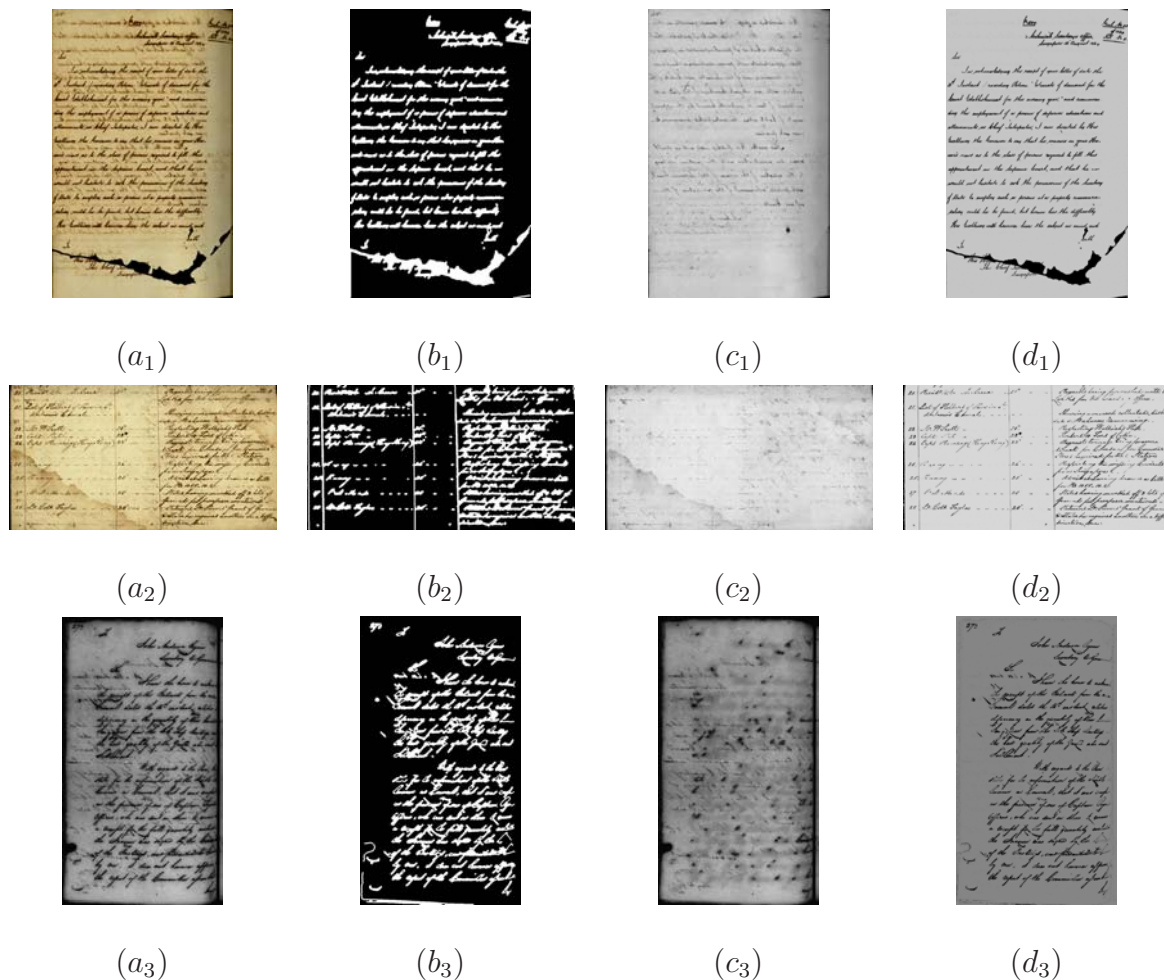
Figure 3.6: Restoration results of real degraded historical document images with background noise: ( a_1 - a_3 ) Original distorted image; ( b_1 - b_3 ) Extracted inpainting mask; ( c_1 - c_3 ) Reconstructed background layer image; ( d_1 - d_3 ) Restored image.
