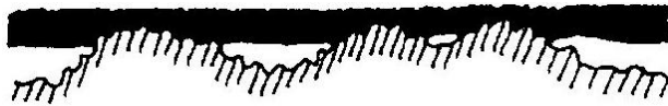
Figure 2.5 Rubber Sliding on a Hard Substrate of Short-ranged and Long ranged Surface Roughness (Persson, 1998)
