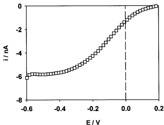
FIGURE 6 Linear sweep voltammogram for the reduction of oxygen at a  $25\text{-}\mu\text{m}$ -diameter Pt UME in a solution containing  $5 \times 10^{-3}\text{ mol dm}^{-3}$  ( $\text{K}_4\text{Ru}(\text{CN})_6$ ) and  $0.2\text{ mol dm}^{-3}$  potassium chloride, phosphate-buffered to  $\text{pH } 7.0 \pm 0.2$ , recorded at a scan rate of  $20\text{ mV s}^{-1}$ .
