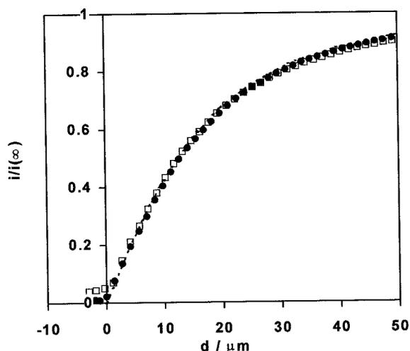
FIGURE 5 Approach curves of normalized current versus sample-tip separation for the diffusion-controlled oxidation of  $\text{Ru}(\text{CN})_6^{4-}$  at a  $25\text{-}\mu\text{m}$  diameter Pt UME approaching cartilage ( $\square$ ) and a flat glass surface ( $\bullet$ ). The dashed line represents the theoretical response for approach to an impermeable substrate (Kwak and Bard, 1989).
