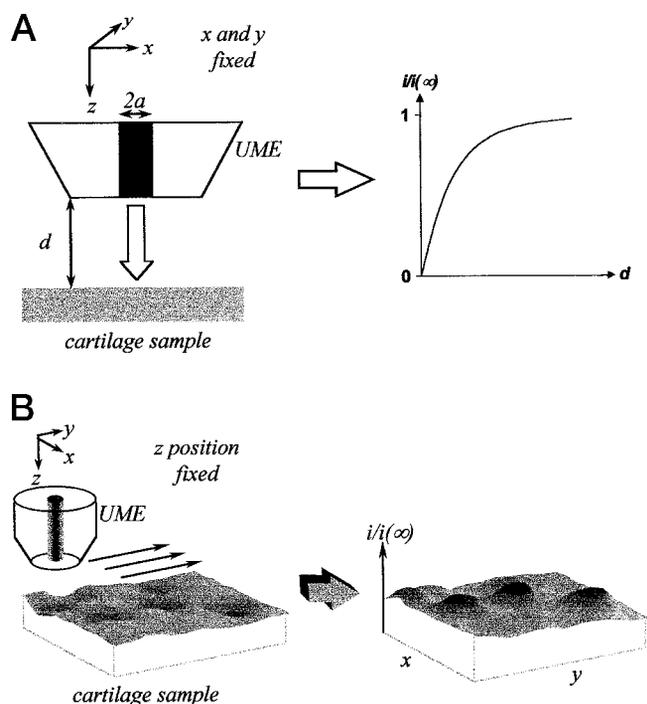
FIGURE 1 Schematics depicting the different modes of SECM operation for (A) tip approach measurements and (B) imaging experiments (not to scale).
