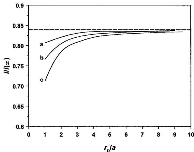
FIGURE 14 Simulated normalized steady-state current as a function of normalized pit radius ( $r_p/a$ ) for  $\gamma = 0.5$ ,  $K_e = 1$ , and a distance  $d/a = 0.8$ . Normalized pit depths,  $d_p/a$ , take the values (a) 0.2, (b) 0.4, (c) 0.6. The dashed line represents the steady-state current predicted for a UME at a distance  $d/a = 0.8$  above a planar surface.
