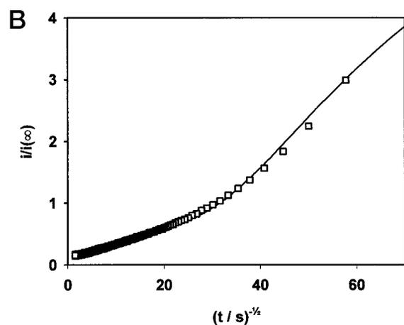
FIGURE 10 Plots of  $i/i(\infty)$  vs. (A)  $t$  and (B)  $t^{-1/2}$  for the diffusion-controlled oxidation of  $\text{Ru}(\text{CN})_6^{4-}$  at a 5- $\mu\text{m}$ -diameter Pt UME recorded at  $d = 0.6 \mu\text{m}$  from the cartilage surface ( $\square$ ). The theoretical response for an impermeable substrate with the tip at a  $\log(d/a)$  of  $-0.6$  is also shown (—).
