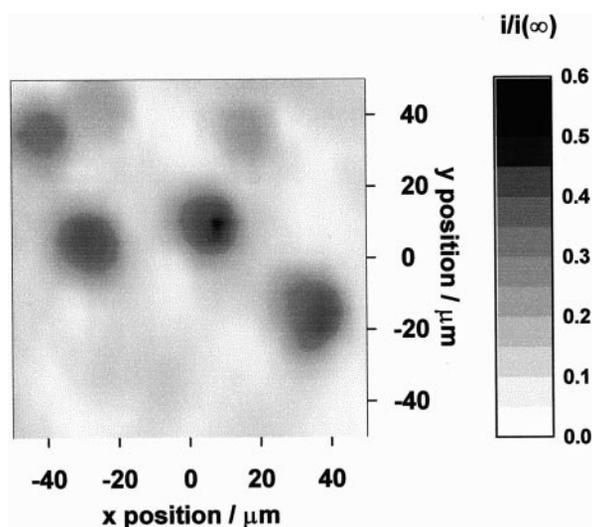
FIGURE 8 Contour plot showing the normalized current map for a  $100 \times 100 \mu\text{m}$  area of cartilage, imaged using the diffusion-controlled oxidation of  $\text{Ru}(\text{CN})_6^{4-}$  at a  $5\text{-}\mu\text{m}$ -diameter Pt UME at an initial sample-tip separation of  $\sim 2 \mu\text{m}$ .
