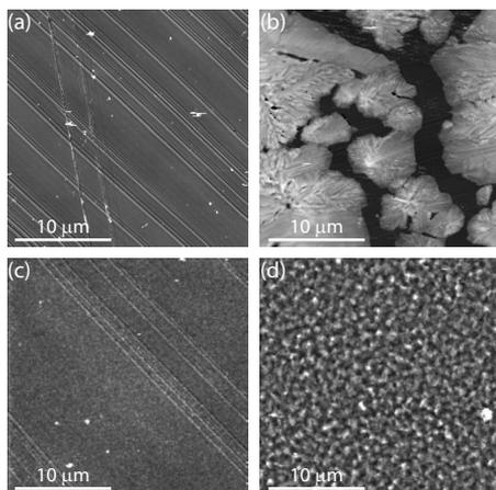
FIG. 2. 25  $\mu\text{m}^2$  AFM micrographs of the MBE Ge layers deposited on 4H-SiC (a) HD-Ge, 300°; (b) HD-Ge, 500 °C; (c) *i*Ge, 300 °C; and (d) *i*Ge, 500 °C. The height scales are [(a) and (c)] 25, (b) 1.25, and (d) 250 nm.
