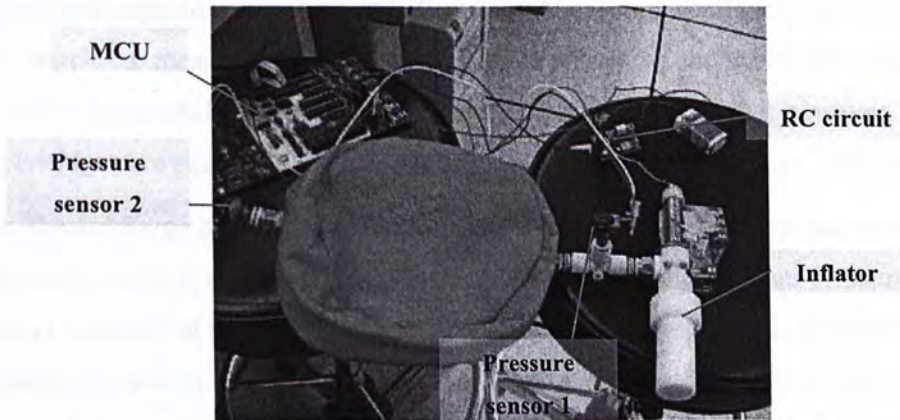
Figure 4-29) The setup for measuring the airbag pressure inflated by the inflator
