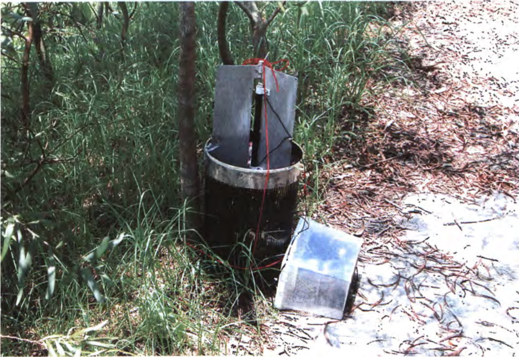
Plate 5.1 A light trap consisted of five components: a blacklight lamp, three baffles around the lamp, a funnel, a holding container and a portable power supply.
