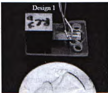
Figure 2.3: Photograph of Roundy's piezoelectric generator (Design 1) [40]. Photo courtesy of Shad Roundy
