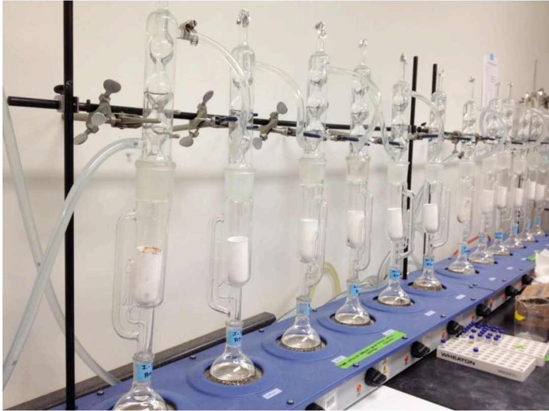
Figure 2. Photograph of Soxhlet tissue extraction system that was used to extract organic pollutants from the liver of barred sand bass.
