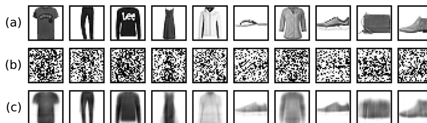
Fig. 3 Example images for the denoising task. Row a contains original images from the Fashion-MNIST dataset. Row b shows the same images with additional Gaussian noise. These noisy images serve as input data for the trained system. Row c shows the obtained reconstructions of the original images.
