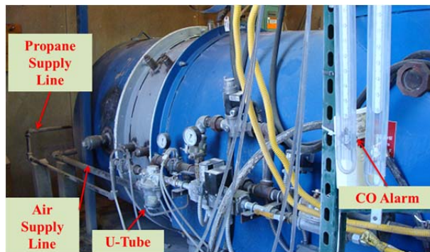
Figure 19. Propane and Air Supply Lines into the Bench-Scale SAP Reactor.
