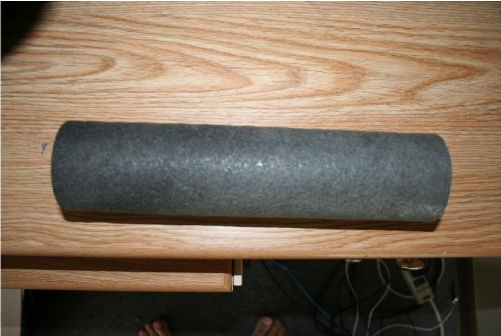
Figure 17. Claris Series filter from the Pall Corporation (a) after 1550 ppm graphite-ethanol suspension run and (b) after 1000 ppm CNT-ethanol suspension run.
