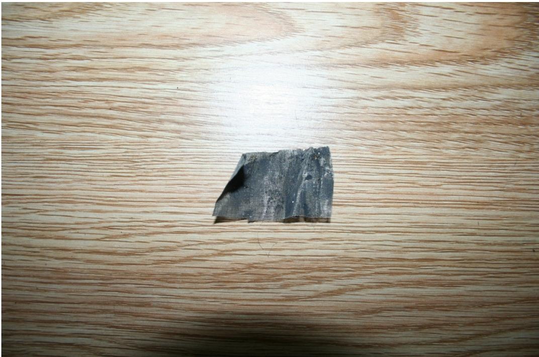
Figure 19. Mesh screen filter from McMaster-Carr after 1000 ppm CNT-ethanol suspension run (a) intact and (b) cut open and laid flat.
