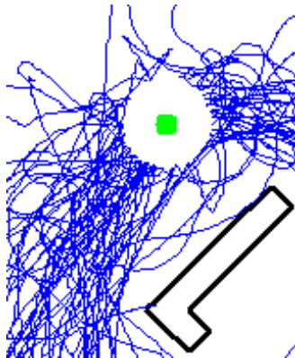
Figure 7.1 Once an operator drives closer to the goal than the threshold, the trial is terminated and considered a success.
