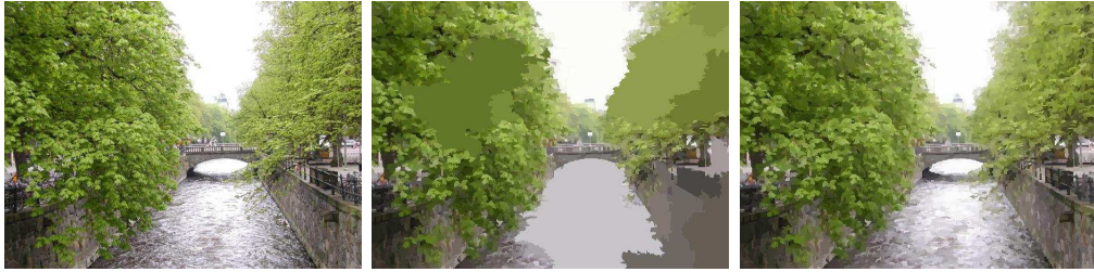
Figure 7: Optimal Cuts for texture using variance of chrominance for scale \lambda = 100 : Left, input Image, middle and right, cuts for parameters at \mu = 10^{12} (low uniformity) and \mu = 10^{14} (high uniformity), in Eq. 22.
