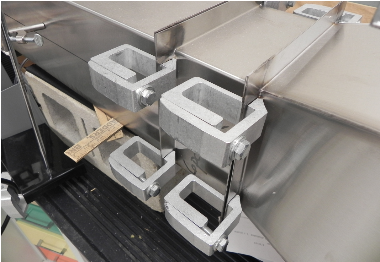
Figure 3.4: Three sections of the Bio-TEC coupled with clamps. The flanges are gasketed with a closed cell foam material
