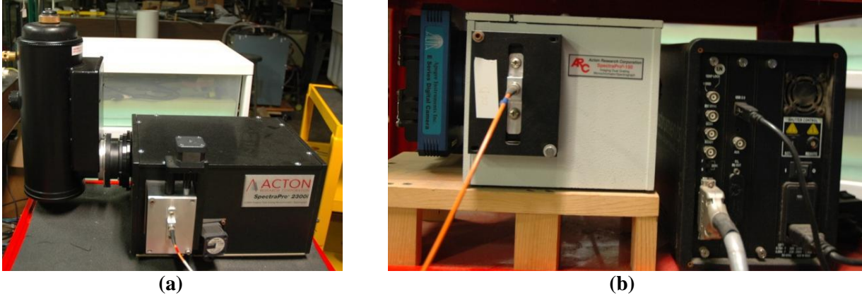
Figure 2.2. (a) OMA used to take measurements of O_2(a) emission at 1268 nm and (b) CCD used to take measurements of O_2(b) at 768 nm. Both OMA and CCD are fiber-coupled, increasing measurement flexibility. The OMA has a collimator that attaches to the diagnostic block during experiments.
