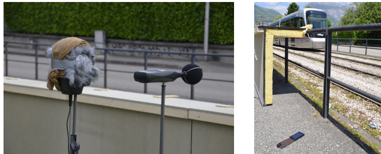
Figure 6: Devices used in the measurements. Left: B&K type 2250 sound level meter and binaural head. Right - cellphone LG P970 used as an auxiliary microphone for speed measurement.
