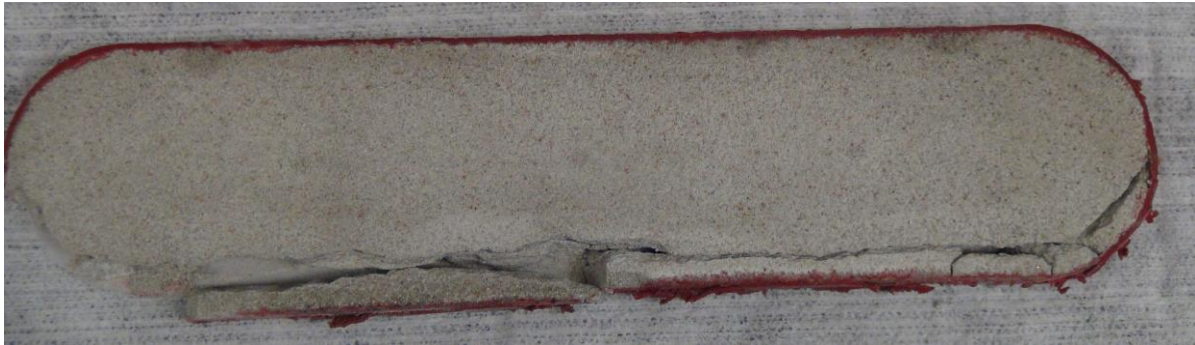
Figure 2: Sandstone Platen Shear Failure
