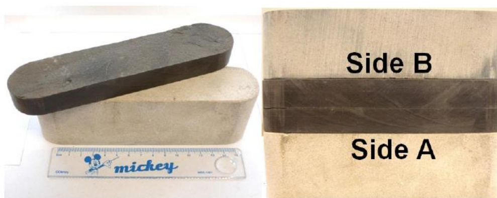
Figure 20: Barnett shale samples shaped to fit into modified API conductivity cell (Zhang, et al. 2013)
