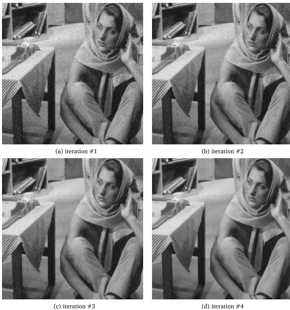
Figure 10: Results obtained at each iteration of the algorithm ( N_{\Delta} = 4 ) when applied to the noisy (WGN) barbara 512 \times 512 image ( \sigma = 20 ).
