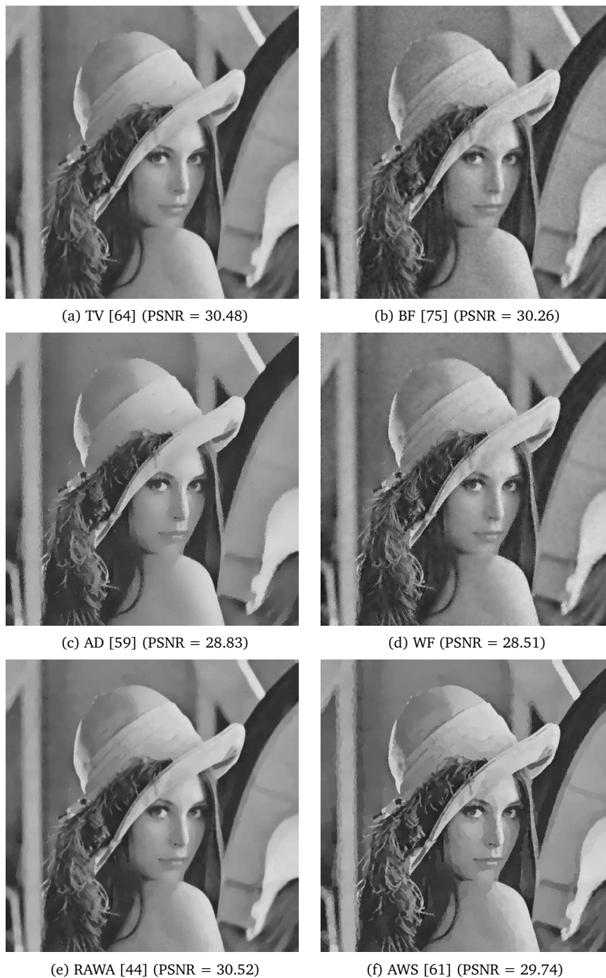
Figure 4: Comparison with restoration methods applied to the noisy (WGN) lena image ( \sigma = 20 ): (a) Total Variation (TV) minimizing process [64], (b) bilateral filtering (BF) [75], (c) anisotropic diffusion (AD) [59], (d) Wiener filtering (WF), (e) adaptive weights smoothing (AWS) [61], (f) robust adaptive window approach (RAWA) [44].
