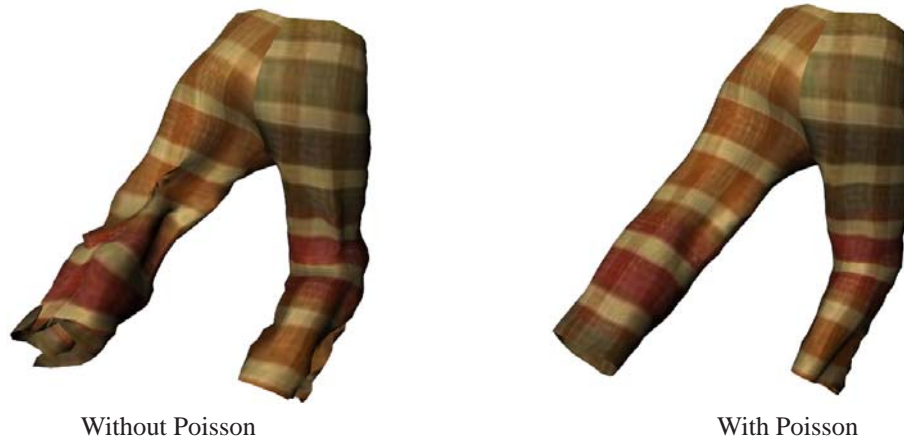
Figure 2.5: Deformation prediction without an additional translation solver may yield distorted results. However, once our Poisson-based translation solver has been applied, the resulting deformation becomes natural without artifacts.
