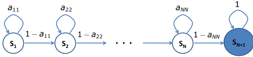
Figure 6.1: The underlying state diagram of a transient HMM with a left-to-right topology and a final non-emitting absorbing state.
