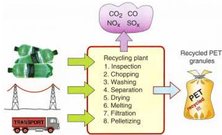
Figure 3.4 Recycling from “Materials and the Environment”: many steps are involved, all of which consume some energy, but the embodied energy of the material is conserved. (Ashby, 2009)
