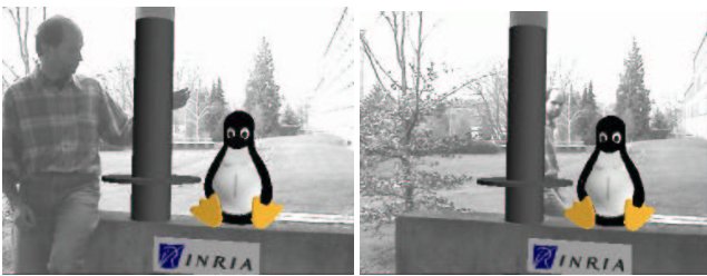
Figure 6. Tracking considering a cylinder and two straight lines with application to augmented reality.
