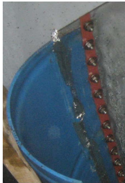
Figure 4.27: (L) Oil test tank assembled inside blast tank (R) Oil test tank seals
