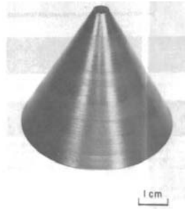
Figure 2.1: Stratified Ni/Cu liner formed by Walters and Golaski [1]
