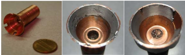
Figure 3.7: (Left) Copper piece before pouring (Center) Trial 1 after machining (Right) Trial 2 after machining
