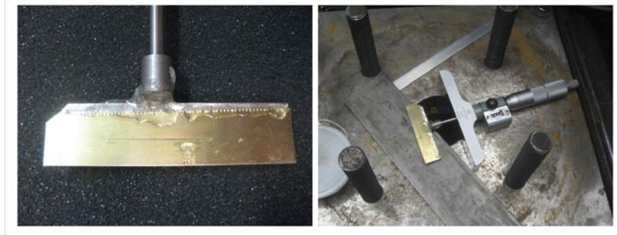
Figure 4.23: (L) Laser line measuring attachment with 100 \mu\text{m} slit (R) Magnetic attachment to depth micrometer
