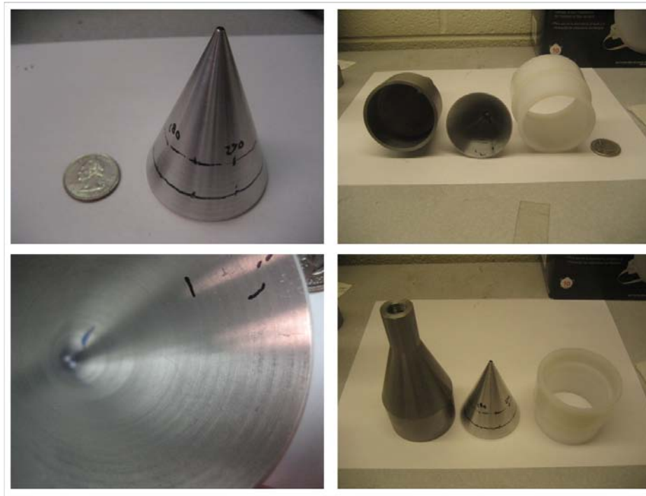
Figure F.6: Pictures of solid copper liner, 50.75 mm diameter, test 12
