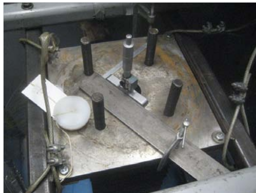
Figure 4.24: Depth micrometer and slit attachment measuring depth of laser lines below base plate
