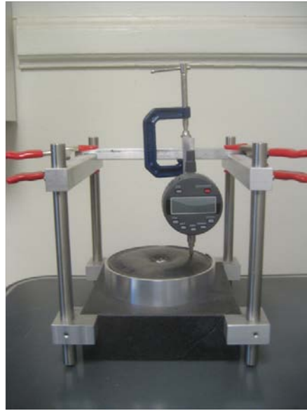
Figure 4.6: Measuring apparatus used to quantify plate deformation for plates from containment tube
