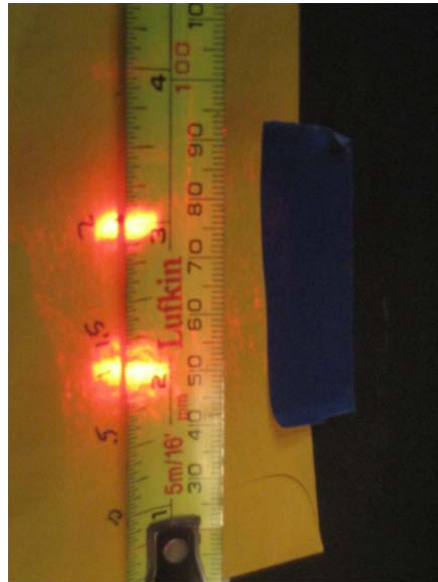
Figure 4.19: Laser line spacing, width, and thickness for test 11
