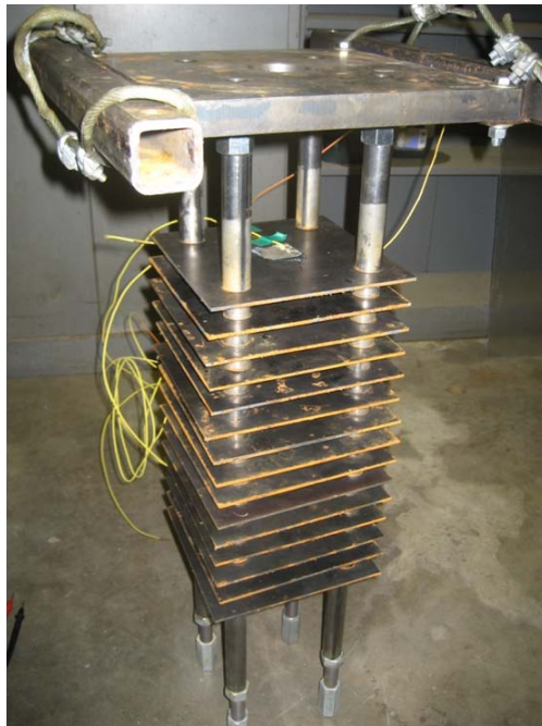
Figure 4.13: Photo showing base plate with attached threaded rods, target plates, spacers, and nuts
