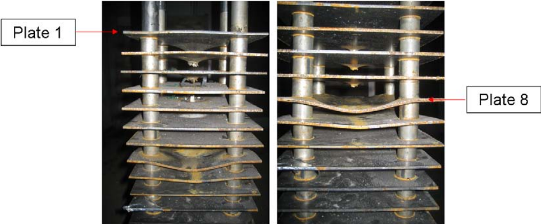
Figure 5.4: Deformation of plates from test 11. In both pictures the plates at the top were nearest the base plate.
