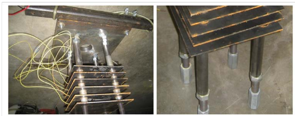
Figure 4.14: (L)Photo showing base plate with threaded rods attached by two 3/4"-10 nuts (R)Bottom of plate array showing compressing spacer, compressing nut, and coupling nut
