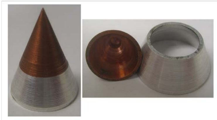
Figure 3.8: (L) Composite liner created using JB Weld ® adhesive (R) Liner separated on the lathe just before achieving the desired thickness
