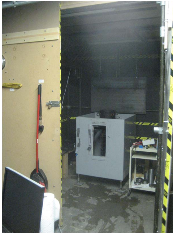
Figure 4.1: Sound enclosure with AcoustiBlok ® sound deadening material
