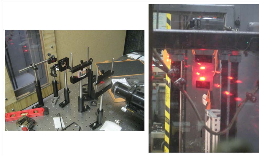
Figure 4.18: (L) Laser velocity diagnostic used for tests 11 - 13 (R) Multiple reflections as the laser passes through the sound enclosure and tank windows
