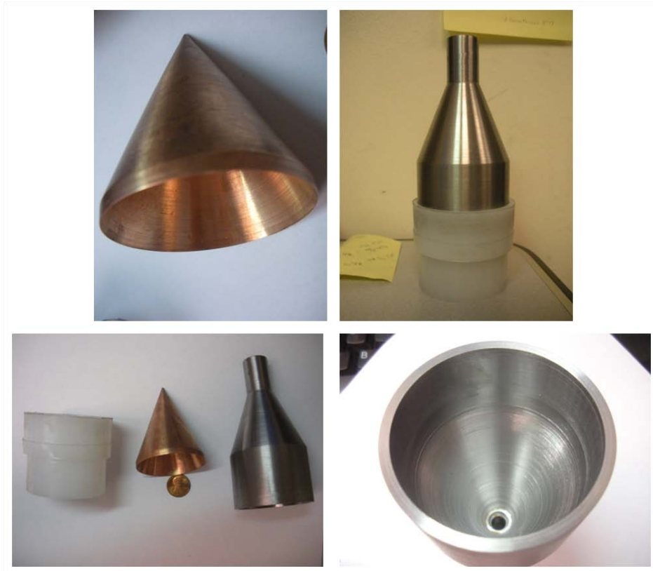
Figure F.4: Pictures of solid copper liner, 50.75 mm diameter, test 10
