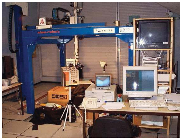
Figure 3.8 – Experimental system: Cartesian robot
