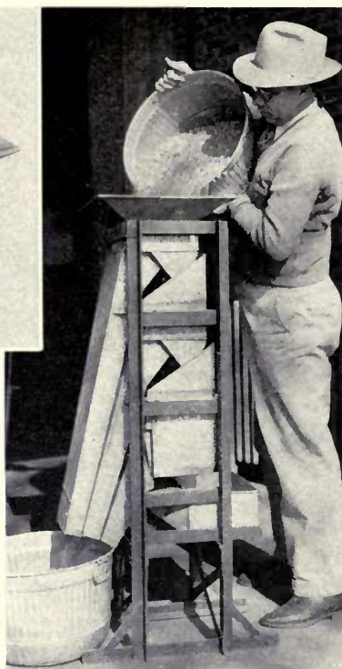
Device for obtaining representative samples of shelled corn. Three similar sets of two-way funnels reduced the lot to \frac{1}{8} original size in the first pouring, and \frac{1}{64} in the second pouring. Detail of the top set of funnels is shown above. (Fig. 19)
