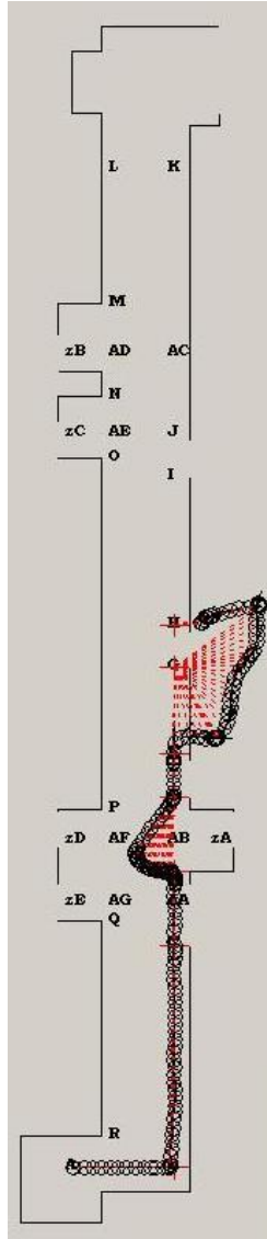
Figure 6.1: This failed run demonstrates that trying hard enough can confuse the robot enough to render it lost. Additional work must be done to deal with this.
