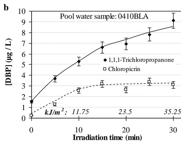
Fig. 3 - Effects of “UV + Cl<sub>2</sub>” pre-treatment ([Cl<sub>2</sub>]<sub>0</sub> = 3 mg L<sup>-1</sup>; Irradiance = 19.5 W m<sup>-2</sup>) on the chlorine demand of a pool water during post-chlorination (Fig. 3a) and on the concentrations of chloroform (Fig 3a) 1,1,1-trichloropropanone and chloropicrin (Fig. 3b) determined after the post-chlorination treatment (Post-chlorination: [Cl<sub>2</sub>]<sub>0</sub> = 3 mg L<sup>-1</sup>, Reaction time = 24 h, 25.0 °C).
