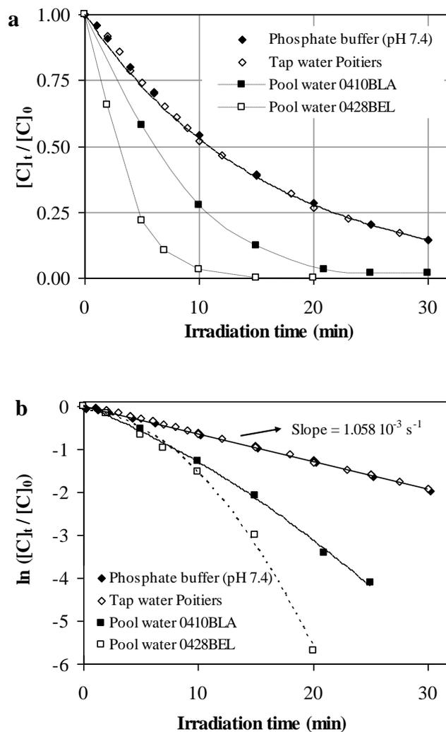
Fig. 2 - Photodecomposition of free chlorine in phosphate-buffered water, tap water and in two pool water samples. a) Concentration time profiles for free chlorine and b): first-order plots for free chlorine decomposition. ( $[\text{Free chlorine}]_0 = 3.0 \text{ mg L}^{-1} = 42 \text{ } \mu\text{M}$ ;  $25.0 \text{ } ^\circ\text{C}$ ; Irradiance =  $19.5 \text{ W m}^{-2}$ ).
