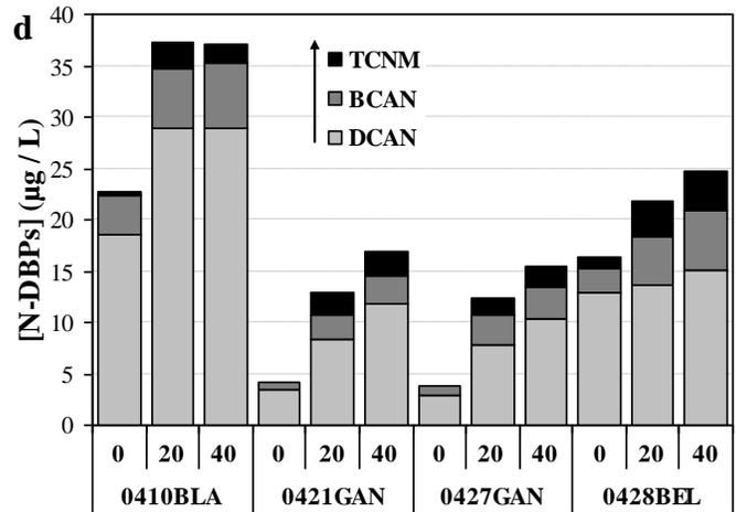
Fig. 4 - Effects of the “UV+ Cl<sub>2</sub>” pre-treatment of four pool water samples on the chlorine demands (a) and on the concentrations of DBPs (b-d) determined after the post-chlorination treatment (UV exposure times of 0, 20 and 40 min corresponding to UV doses of 0, 23.5 and 47 kJ m<sup>-2</sup>, respectively).
