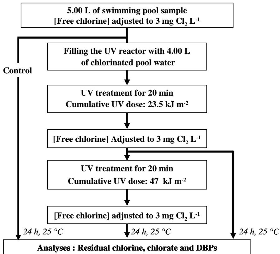
Fig. 1 - Experimental design for UV treatment and chlorination experiments.
