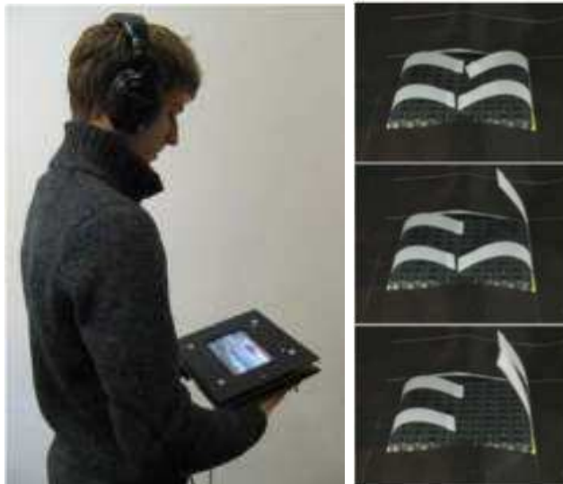
Figure 2.8: Handheld haptic device. A mobile haptic TV embedding an array of ultrasonic transmitters delivering tactile cues on user's fingers [AMS11].
