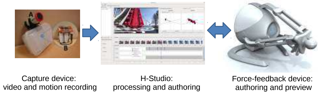
Figure 5.1: Overview of the H-Studio . Video and motion effects can be imported from our capture device, or manually edited thanks to a force-feedback device. This device can also be used to preview motion effects.
