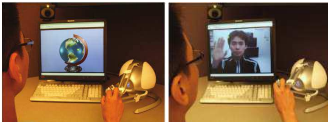
Figure 2.10: Desktop haptic device. User touching a video thanks to a force-feedback device [CES09].
