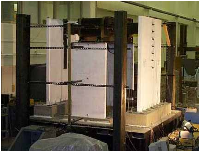
Figure 3-11: ST-10 Test Structure on the Shake Table (out-of-plane URM wall is in foreground)
