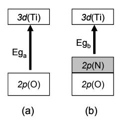
Fig. 2 : Evolution of the optical bandgap from TiO\_2 (a) to nitrogen-doped TiO\_{2-x}N\_x (b).
