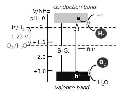
Fig. 5: Schematic of overall water splitting (from Domen et al.)
