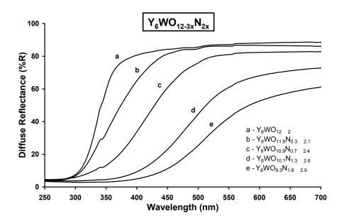
Fig. 3 : Diffuse reflectance spectra in the  $Y_6WO_{12-3x}N_{2x}$  system [24].
