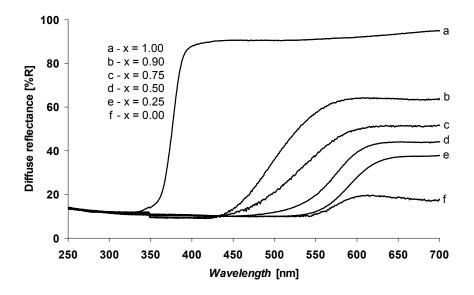
Fig. 4 : Diffuse reflectance spectra of La<sub>1-x</sub>Sr<sub>x</sub>Ti(O,N)<sub>3</sub> compositions [14].
