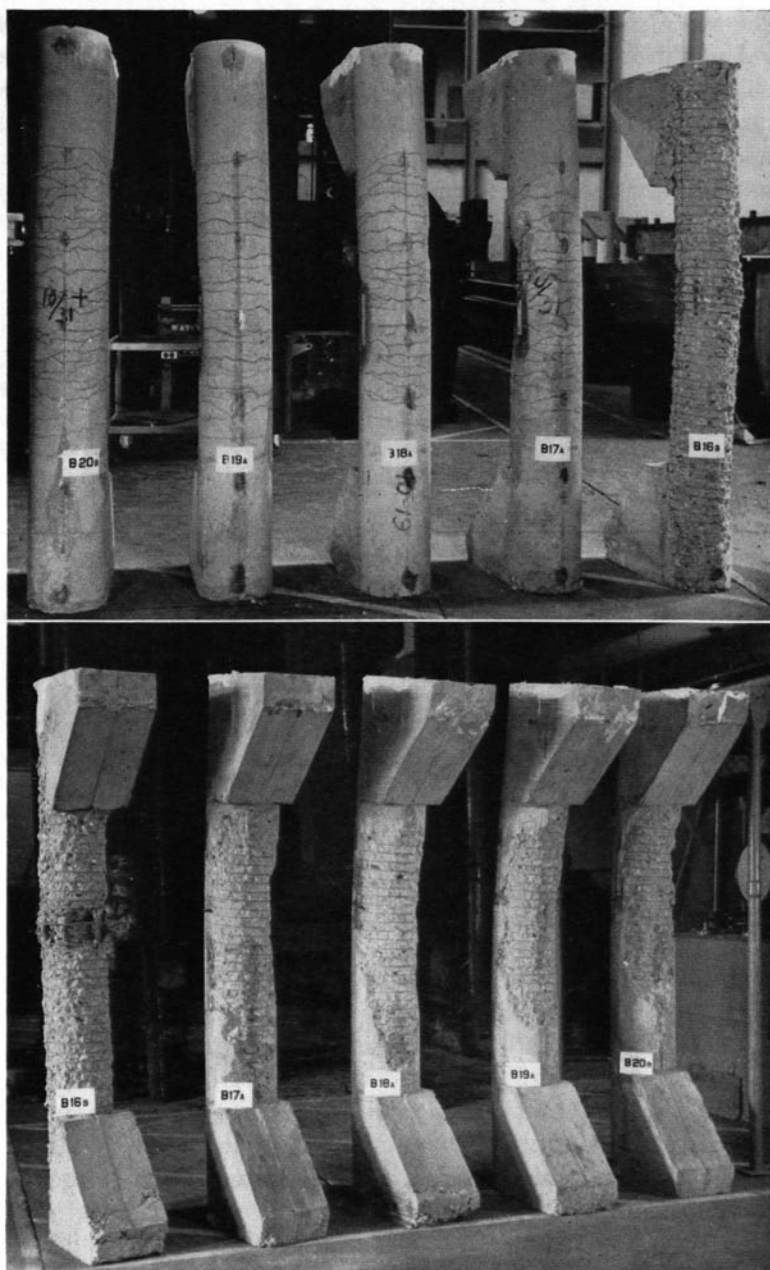
Fig. 39. Columns B-16 to B-20 after Failure
