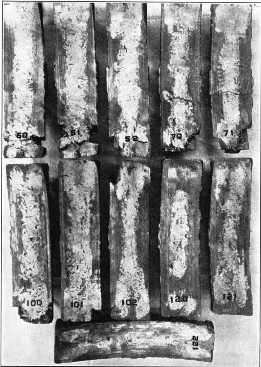
FIG. 9b. CONDITION OF SHOES AFTER TESTS
