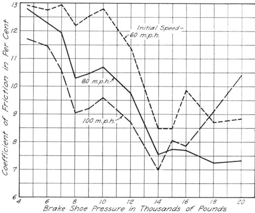
FIG. 1. RELATION BETWEEN COEFFICIENT OF FRICTION AND BRAKE SHOE PRESSURE, FOR ALL TESTS
