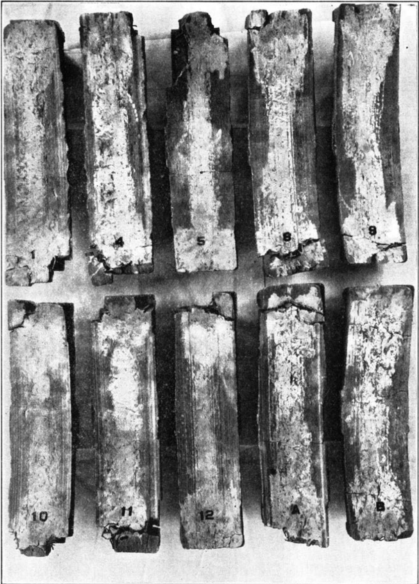
FIG. 9a. CONDITION OF SHOES AFTER TESTS
