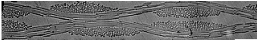
Fig. 5. Photomicrographs of 3313 laminate (110x) a) warp yarns parallel to the page, fill yarns perpendicular, b) fill yarns parallel to the page, warp yarns perpendicular.
