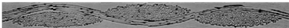
Fig. 6. Photomicrographs of 7628 laminate (67x) a) warp yarns parallel to the page, fill yarns perpendicular, b) fill yarns parallel to the page, warp yarns perpendicular.
