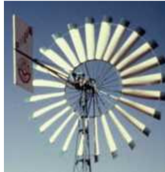
Figure 2: High solidity rotor Photo: Practical Action
