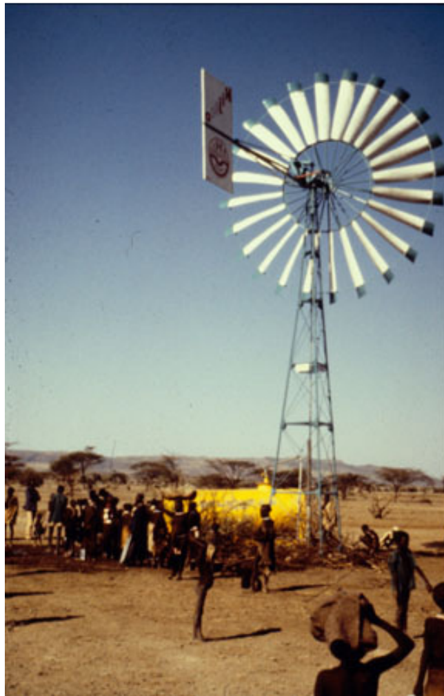
Figure 3: The Kitjito Windpump used to pump ground water in the Bhel region of Turkana for the nomadic pastoralists. Photo: Practical Action.
