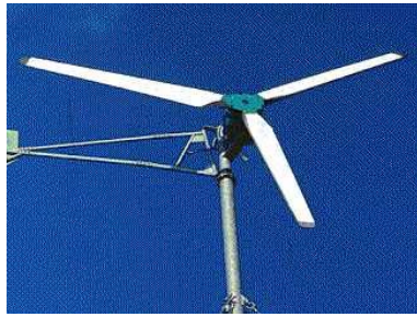
Figure 1: Low solidity rotor Photo: Practical Action
