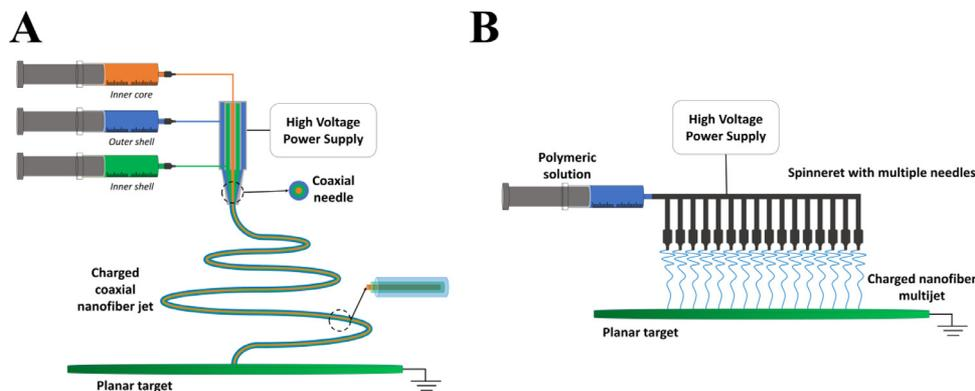
**Fig. 10.** Schematization of advanced electrospinning apparatus. Electrospinning devices can be modified in order to produce tailored membranes; in A) coaxial needles can be used to produce core-shell structured nanofibers using different polymeric solutions for the core and for the shells of the nanofiber. In B) a spinneret with multiple needles is used to speed up the deposition of nanofibers and the production of electrospun membranes.
