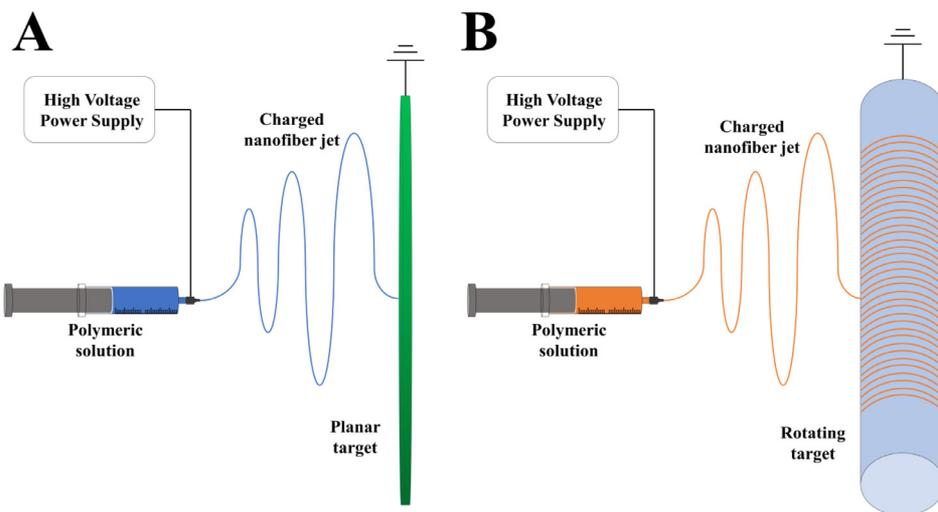
**Fig. 9.** Electrospinning apparatus schematization. The high voltage supply connected both to the spinneret and the collector enables liquid surface tension overcoming at the tip of the needle and fibre deposition. Two types of setup are represented: A) planar target for the preparation of nanofiber-based membranes; B) rotating target (or mandrel) for the preparation of nanofiber-based tubular scaffolds.
