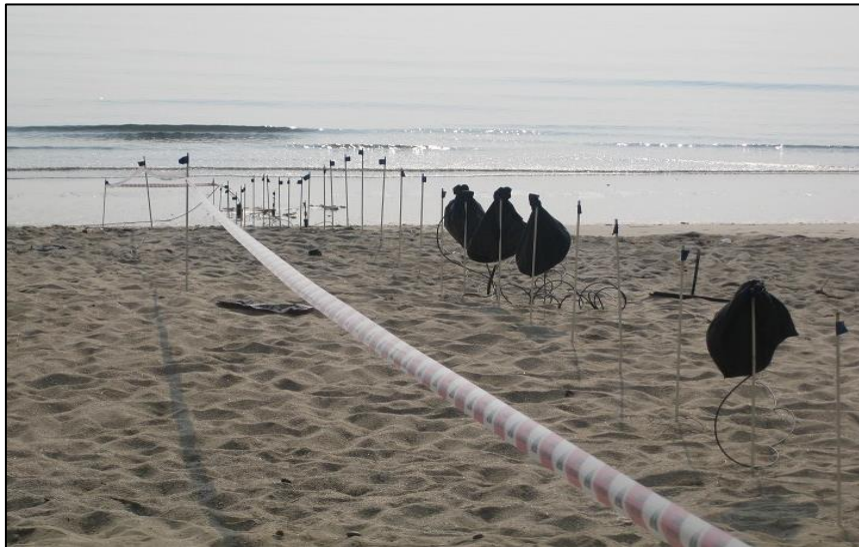
Figure 3.7 A view of the steel rods used for the cross-shore profile measurement
