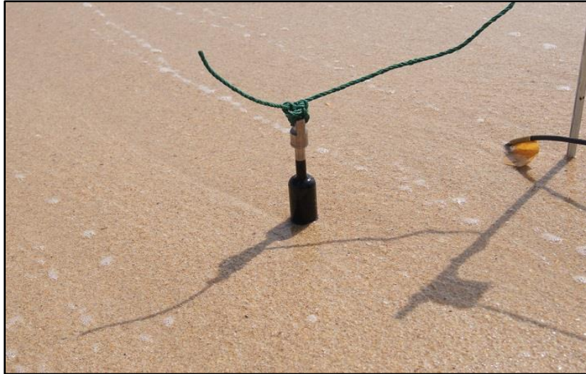
Figure 3.28 The ECM in action for recording the swash flow velocities
