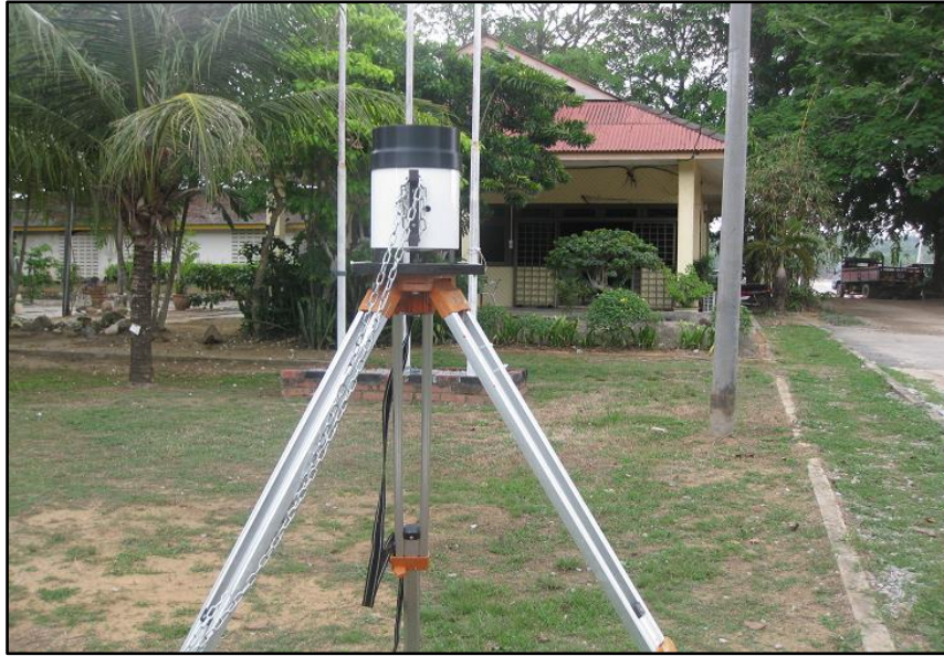
Figure 3.10 Rain gauge installed at the study area
