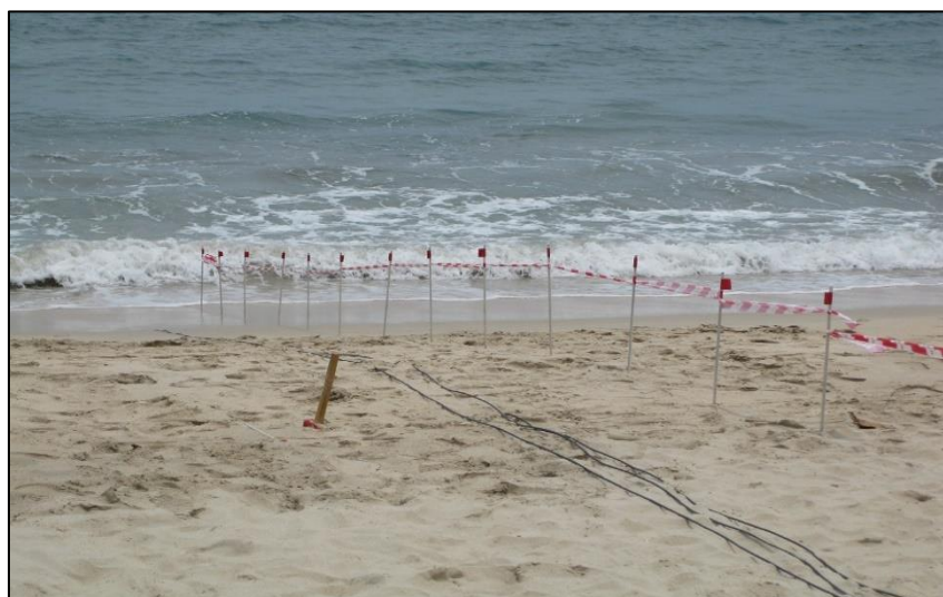
Figure 3.26 Installation of 1-m rod steels along the cross-section
