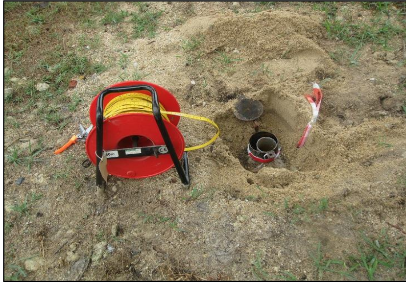
Figure 3.20 Manual reading used for the quality of the groundwater level data
