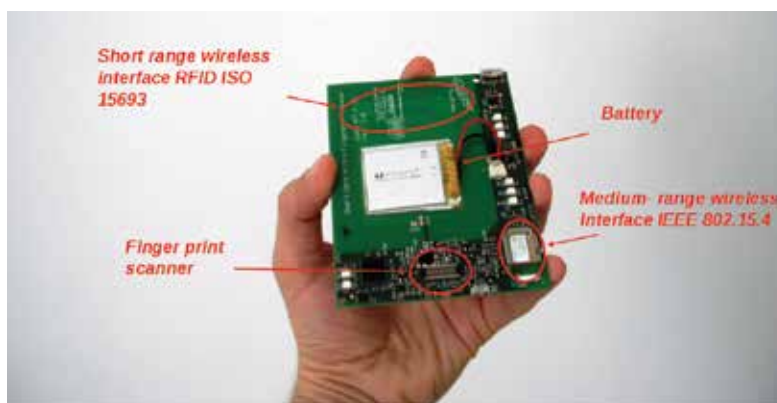
Fig. 2. WEST Aquila's Biometric Badge – components
