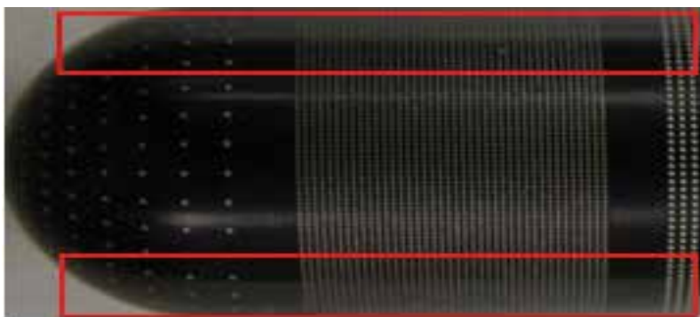
Fig. 3. Image of a test finger taken with a traditional CCD. Distortion in the form of compression and image blur in the top and bottom portions of the image can be seen
