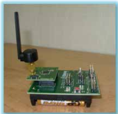
(a) Battery powered anchor node
