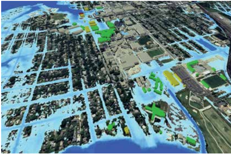
Figure 12. D ortho-perspective of Irene-generated flooding focused on ODU with 3-D building models extruded for perspective. Blue shades depict inundation depth (as described in Figure 5).
