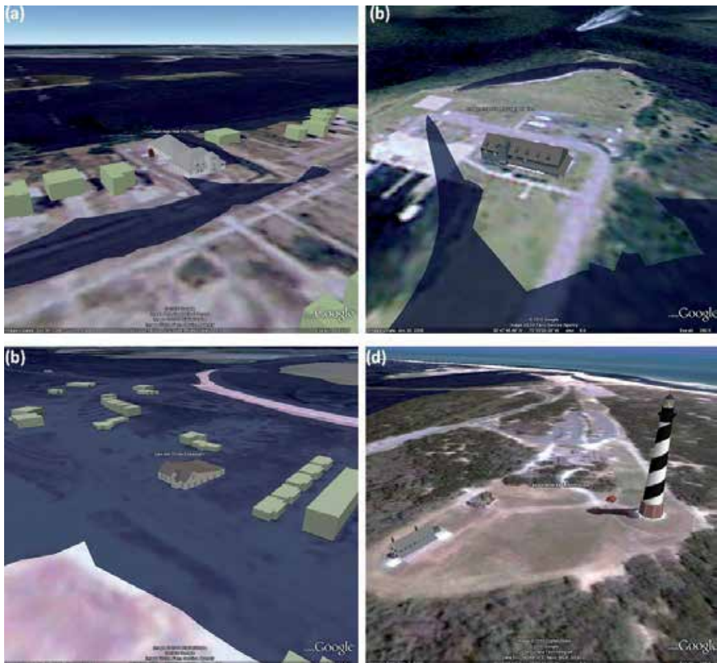
Figure 5. Screenshots of customized.kmz files with building footprint models, landmark 3-D buildings, and SLOSH MOM output storm surge inundation layers superimposed over Google imagery for a category 2 storm affecting the Outer Banks, North Carolina, (a) South Nags Head fire station, (b) US Coast Guard Oregon Inlet station, (c) Sam & Omie's Restaurant at Whalebone Junction, South Nags Head, and (d) Cape Hatteras Lighthouse, Buxton.
