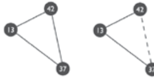
Fig. 8. The SLO-T triangular elimination under unit link cost. The link connecting routers with the highest ids, 42, 37 in the picture, is excluded.
