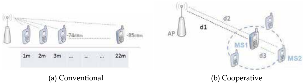
Fig. 15. Conventional and Cooperative calibration for multiple devices.
