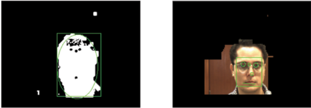
Fig. 4. Skin color detection using depth information.
