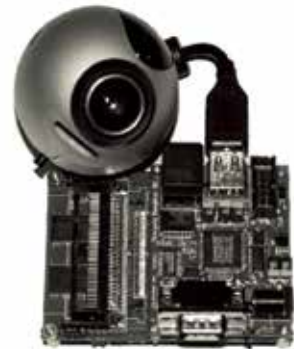
(c) The Crossbow Stargate platform with an attached webcam (Feng et al., 2005).
