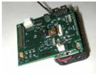
(b) Cyclops with an attached MICA2 node (Rahimi et al., 2005).
