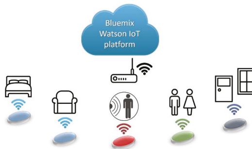
Figure 1. CARDEA (Computer-Aided, Rule-based Domestic Environment Assistant) Wi-Fi system architecture. IoT = Internet of Things.
