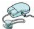
Fig. 12. Possible new mechanical design of the internet tele-stethoscope, alternatively to the classical chassis
