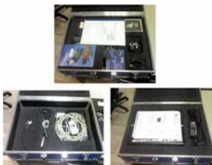
Fig. 26. The remote medical visit system, prototyped for experimental validation, assembled in a small suitcase
