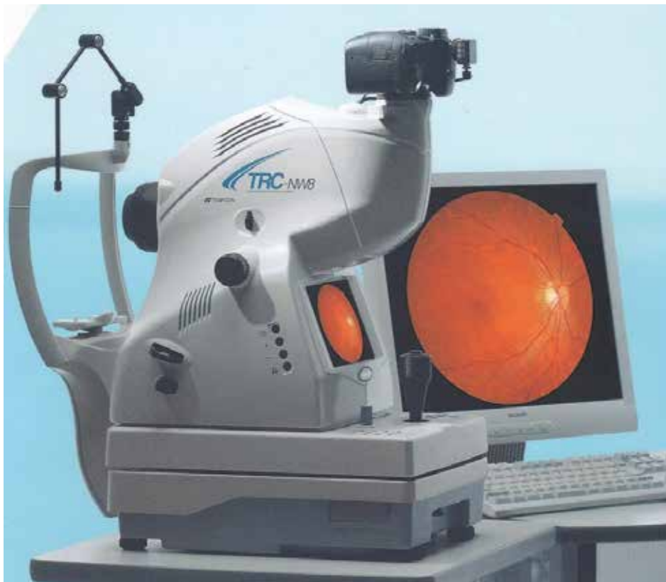
Fig. 2. Digital fundus camera. (Topcon)
