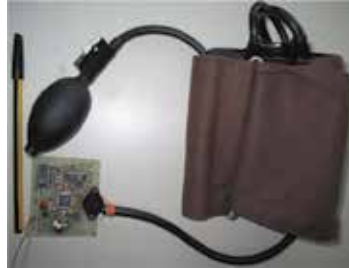
Fig. 29. Prototype of the arterial pressure measurement instrument, PC-based and wi fi connected to PC
