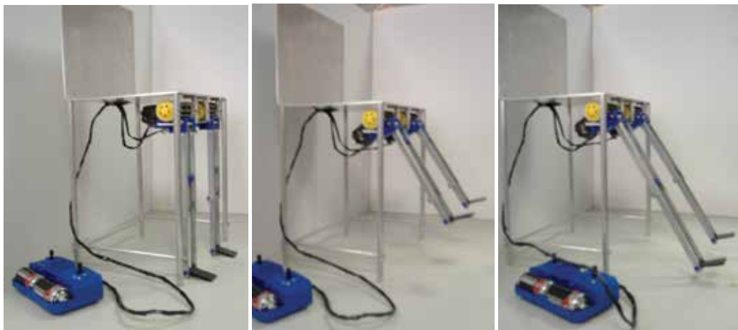
Fig. 23. Motorized foot rest at stationary position Fig. 24. Motorized foot rest after swing angle adjustment Fig. 25. Motorized foot rest after length adjustment
