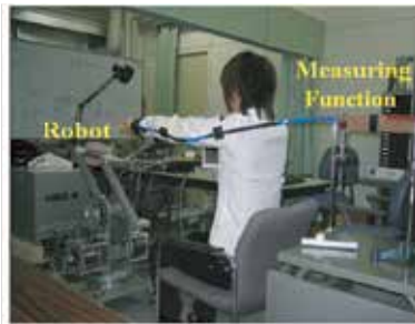
Fig. 1. 3-Dimensional rehabilitation training robot for upper limbs with measuring function
