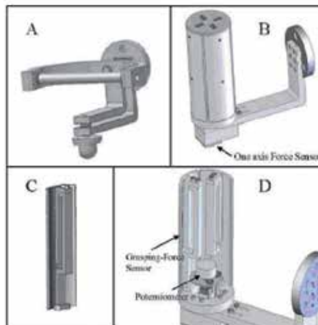
Fig. 34. Sensor grip device: (A) Former handle (passive gimbal), (B) Current handle (sensor grip), (C) A part of grip force sensor, (D) inner mechanism of the grip device
