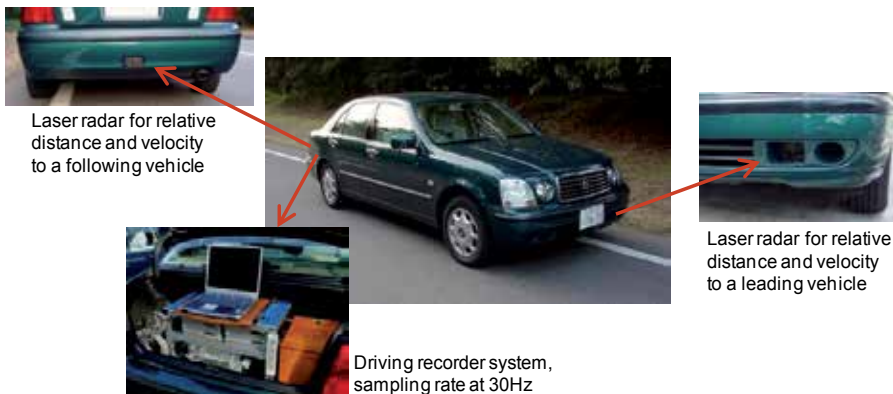
Fig. 3. AIST instrumented vehicle with sensors and a recorder system for detecting nearby vehicles
