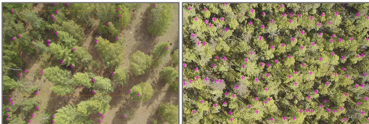
Figure 8.49: Template matching procedure applied for tree count. In both images (UAV image of mission 1 - left; image of mission 007 – right) trees are either correctly identified, falsely designated, or completely missed.
