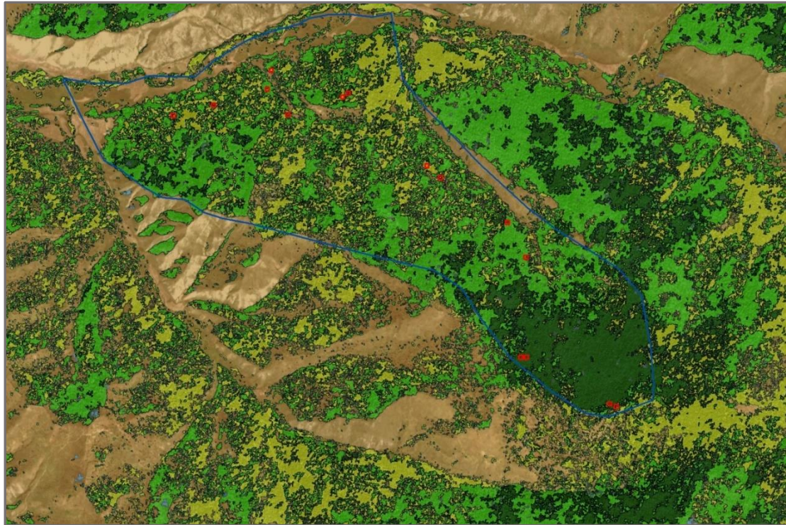
Figure 8.60: Object-based classification of Pléiades image (10/05/2015). Random Forest ( RF ) classifier for dominant tree species classification was used. Classes depicted in graph: birch (yellow), light taiga (bright green), dark taiga (dark green), and grassland/soil (brown).
