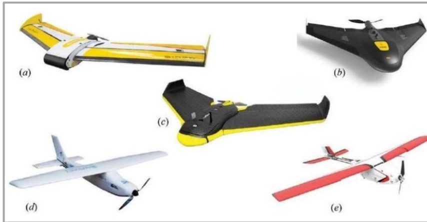
Figure 6.2: Examples of a fixed-wing UAV design: (a) QuestUAV Q-Pod; (b) SenseFly eBee; (c) Trimble UX5; (d) MaVinci Sirius Pro; (e) PrecisionHawk Lancaster (source: Padua, 2017).
