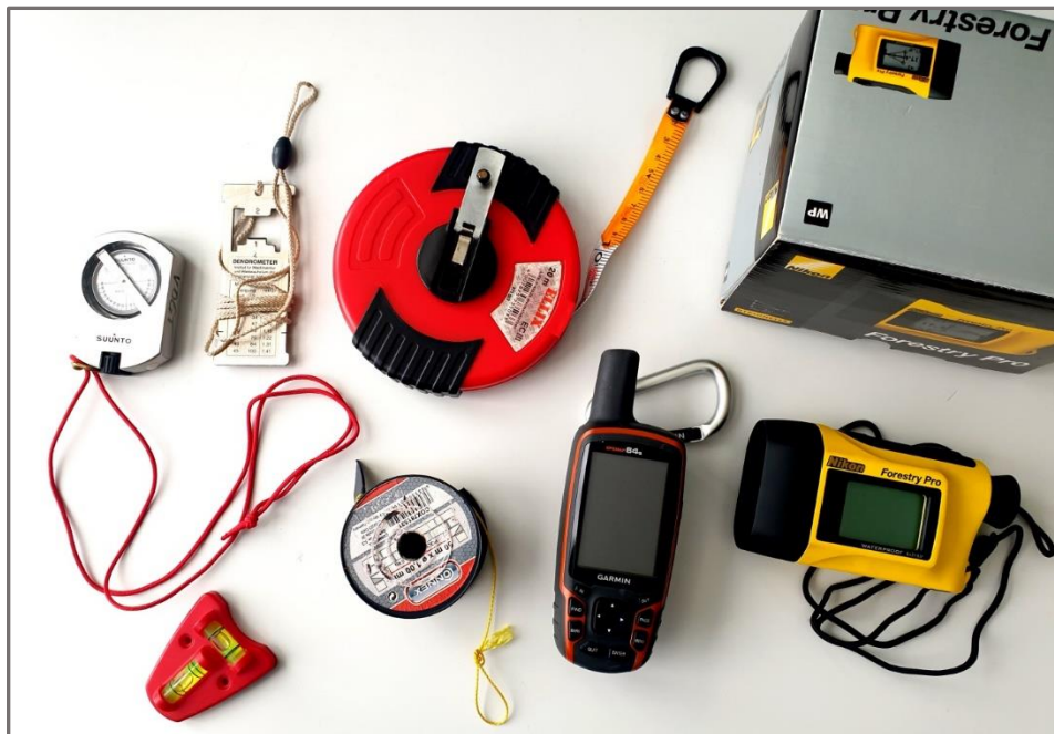
Figure 7.10: Field equipment (selection). Starting from top left: Suunto inclinometer, Kramer dendrometer, measuring tape; bottom left: bubble level, lacing cord, Garmin GPSmap 64s, Nikon Forestry Pro laser rangefinder.
