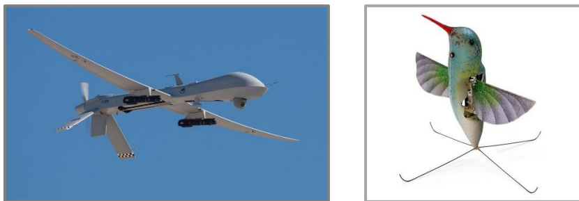
Figure 6.1: Example for a HALE UAV (General Atomics MQ-1 'Predator' - left) and a NAV (AeroVironment 'Hummingbird' - right). Source: manufacturer's photos.
