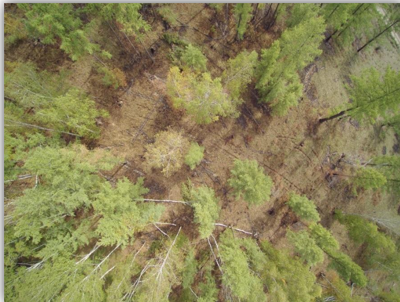
Figure 4.26: The tree at the image centre is rendered perpendicularly, whereas trees further away feature an oblique view (image taken by Vogt, 2017).
