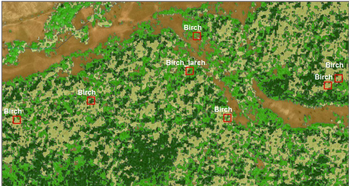
Figure 15.1: Example of misclassification on a Pléiades image (10/05/2015). The red boxes indicate the test plot boundaries, the labels the dominating tree species as found in the field. In some cases, the class birch was misclassified as light or even dark taiga (RF classifier).
