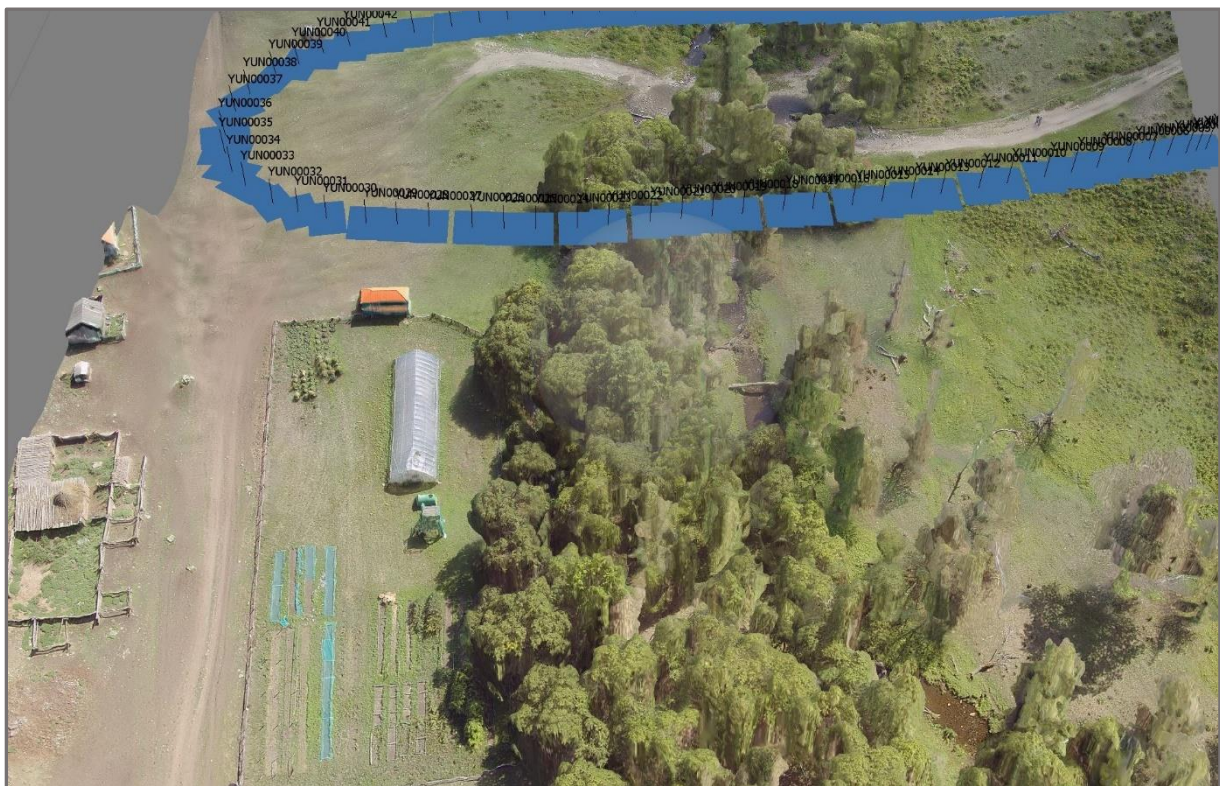
Figure 7.24: Example of a resulting high-resolution 3D model of flying mission 14 (riparian area). The photo locations are indicated with blue squares hovering above the scenery. All features in the model seem precisely represented, especially non-tree objects.
